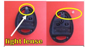
Next you will be separating old button pad from plastic shell. Please note small light lense located at the top of the button pad. You will have to remove it first before detaching
