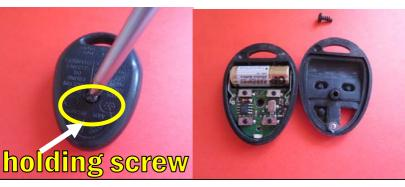
Unscrew a small screw at the back of plastic shell. Open remote and separate top hard shell part with button key pad and part with electronic board and battery. Part with electronics will remain untouched and you will be only working with half of the shell consisting of key buttons.
