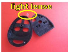
You can lift light lense using small flat screwdriver of just a finger nail. Try not to misplace it as it will be fitted in exactly the same spot once new pad is installed.
